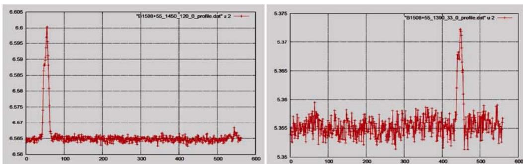
**Figure 5.** Comparison of sample pulsar observations at the L-band from the uGMRT system (using 200 MHz bandwidth of band-5; left panel) with the legacy GMRT system (using 32 MHz bandwidth; right panel) for PSR B1508 + 55, carried out simultaneously with the same set of eight antennas for 10 min, illustrating the improved sensitivity of the uGMRT system.
