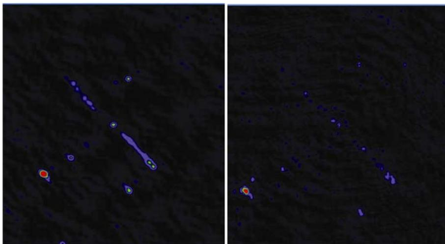
**Figure 4.** Comparison of sample continuum imaging results at the L-band from the uGMRT system (using 250 MHz bandwidth of band-5 and only 2 h of integration time; left panel) with the legacy GMRT system (using 14 MHz bandwidth and 4 h of integration time; right panel), using the same set of antennas, for a giant radio source illustrating the improved quality of the imaging in terms of lower rms noise (35 vs 50  $\mu$ Jy) and reduced artefacts.
