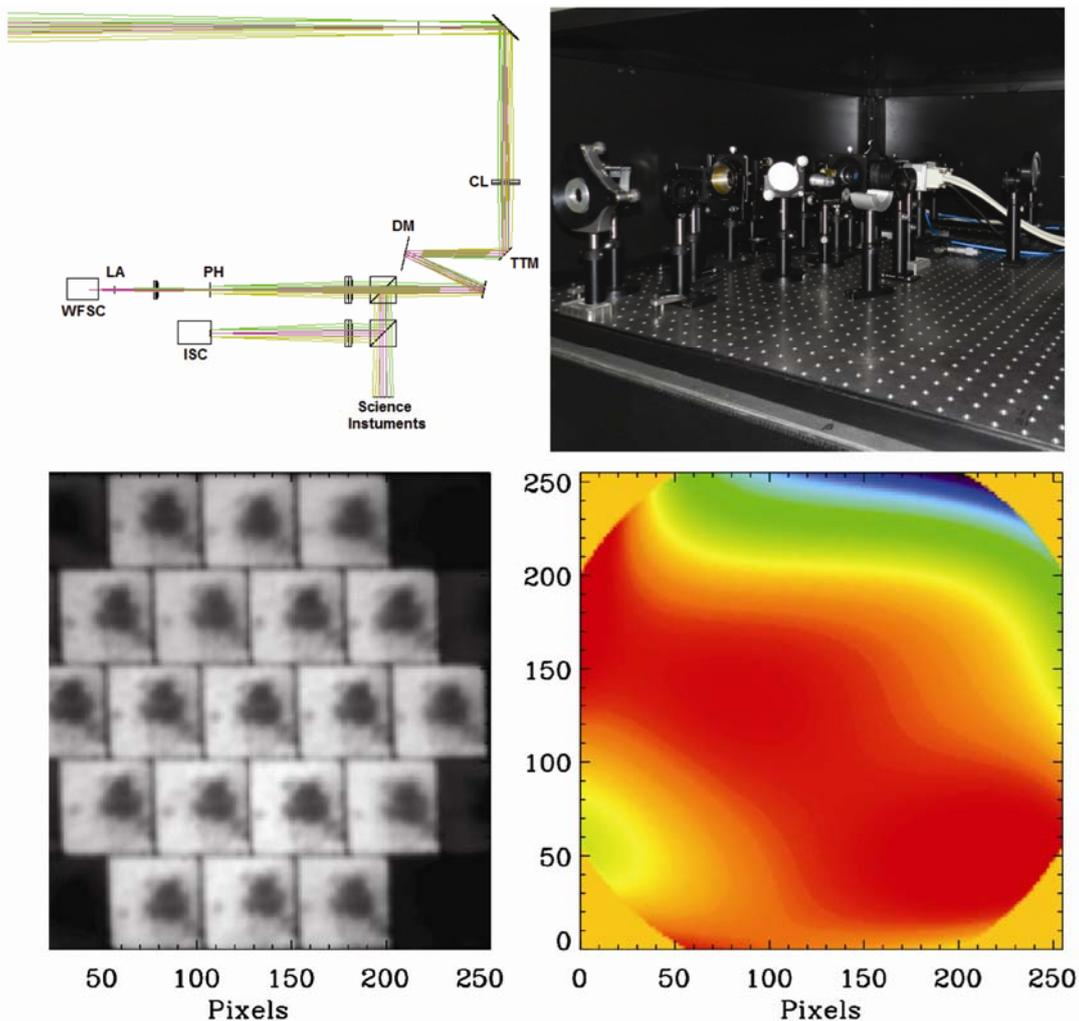
**Figure 4.** (Top left) Optical schematic of the AO system (Top right) The AO system integrated with MAST. (Bottom left) Images from the lens-let array used for calculating the shifts and thus the wavefront distortion. (Bottom right) Wavefront distortion calculated from the shift measurements.
