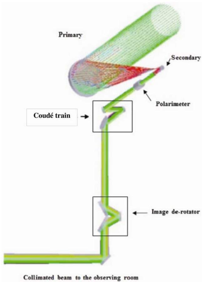
**Figure 1.** Optical layout of Multi Application Solar Telescope (MAST).
