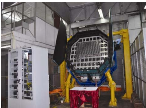
Figure 4. The partially assembled imaging camera of the MACE telescope at ECIL, Hyderabad in June 2016. The central 19 CIM modules can be seen along with the two motorized front shutters. The 48 V power distribution rack connected to the camera can be seen and the left of the photograph.
