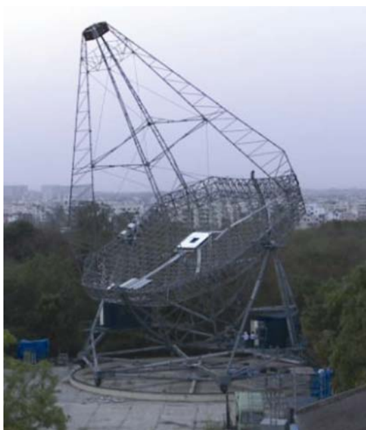
Figure 2. Trial assembly of the mechanical structure of the MACE telescope at ECIL, Hyderabad in June 2014. A set of eight aligned mirror panels can be seen of centre of the mirror basket.
