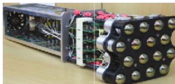
Figure 3. A fully assembled 16 channel camera instrumentation module of the MACE telescope. The 16 photomultiplier tubes can be seen in the front, while the fast signal processing electronics is fixed at the rear of the module.
