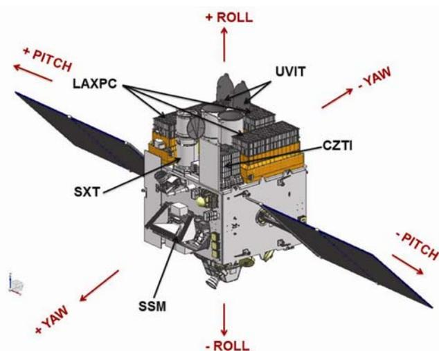
Figure 2. Spacecraft axes definition.
