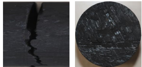
(i) Extension path (ii) Fracture surface (b)
