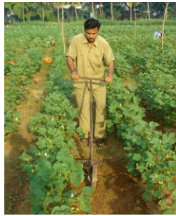
b. Developed weeder
