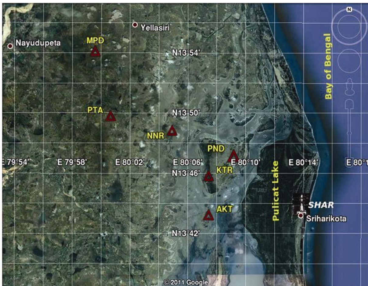
Figure 2. Digital broadband network. Red triangles (MPD, PTA, NNR, PND, KTR and AKT) represent the broadband seismic stations. The white circle represents SHAR, Sriharikota, the point of lift-off of PSLV.
