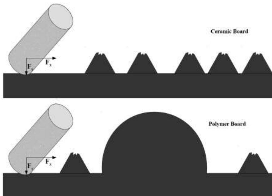
**Figure 7.** Roughness model on the two boards studied. Uniformly spread and densely populated asperities are shown in ceramic board (top), while the polymer board (bottom) possesses sparsely located roughness. Polymer board also possesses abundance of surface waviness, which is described by a large hemisphere.
