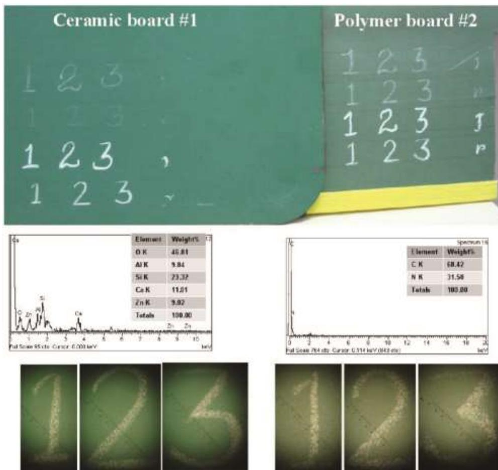
**Figure 4.** Writing performance on two boards, shown in the top image, captured through a camera from a distance of ~1 ft. Numbers 1–3 are written in separate rows and a set of rows is erased to understand the ease of wiping. EDAX profiles of the respective boards and the magnified view, through optical microscope, of numbers written on them are shown in the middle and bottom rows respectively.
