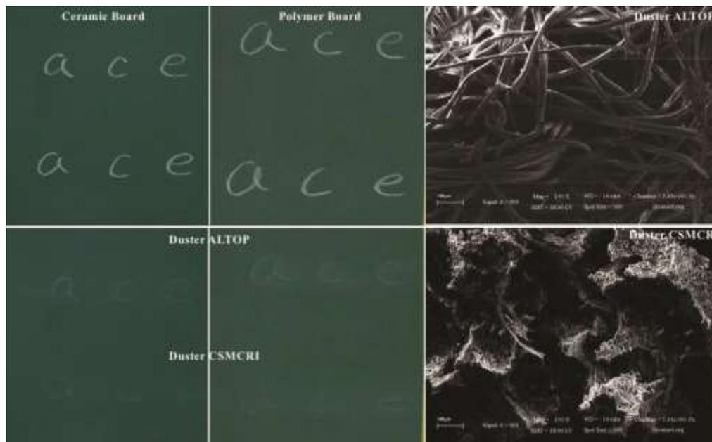
**Figure 5.** Wiping experiment on ceramic (left column) and polymer (middle column) boards using commercially available ALTOP duster (text at the top line) and home-made polyurethane duster (text at the bottom line). SEM images of the dusters are shown in the third column: (top, ALTOP; bottom, CSIR-CSMCRI).
