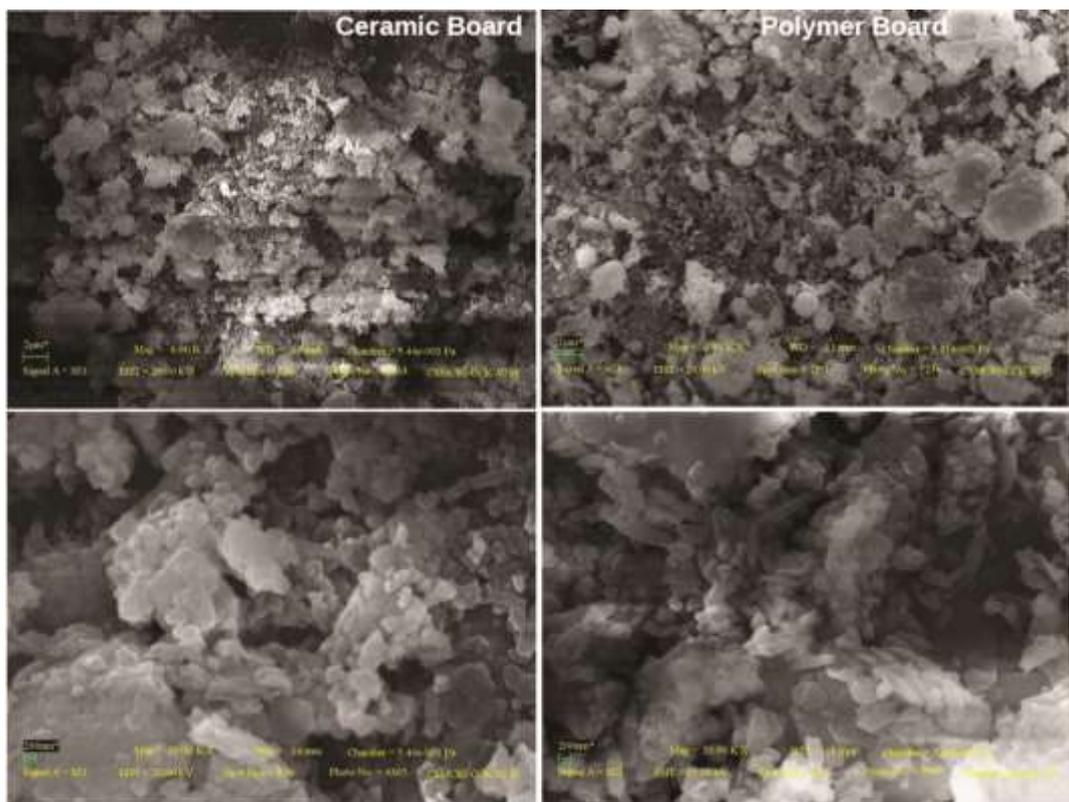
**Figure 3.** SEM images of chalk writing etched on ceramic (left panel) and resin board (right panel) surface. Top row images are acquired at magnification factor of 4000, while bottom row images are acquired at magnification factor of 20,000.
