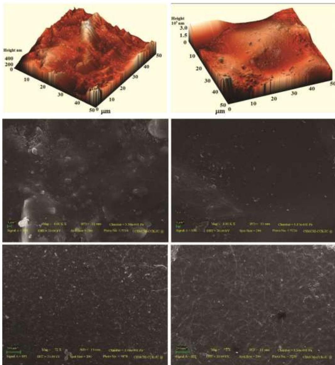
**Figure 6.** Surface topographies of ceramic (left column) and polymer (right column) boards. Top panel compares the topology observed through atomic force microscope. Middle and bottom panels compare the electron microscope images obtained at higher and lower resolution respectively.
