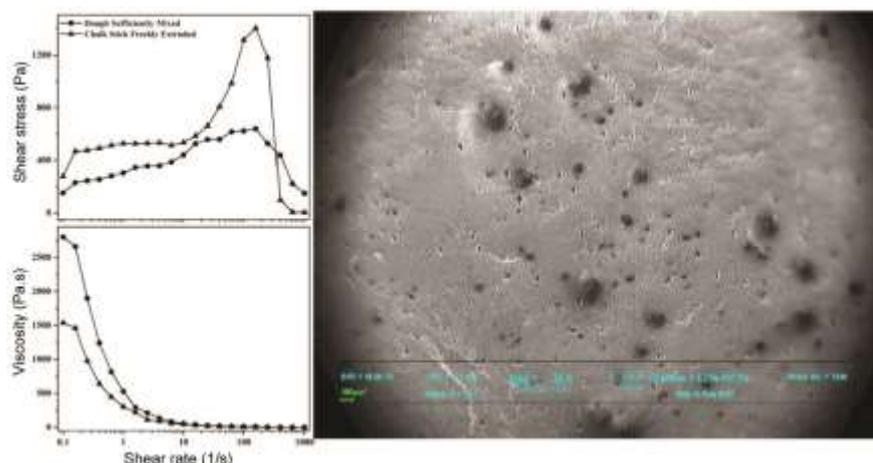
**Figure 1.** (Left) Graphs showing the shear stress and viscosity variation as functions of shear rate for sufficiently mixed dough and the freshly prepared chalk stick. (Right) Low-resolution SEM image of the interior surface of chalk stick exposed after breaking.
