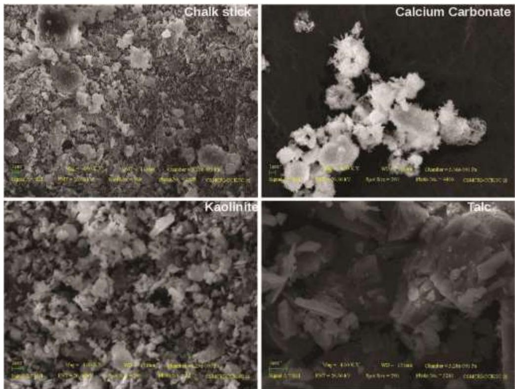
**Figure 2.** SEM images of the chalk stick surface and powders of solid constituents, i.e.  $\text{CaCO}_3$ , kaolinite and talc at a uniform magnification factor of 4000.
