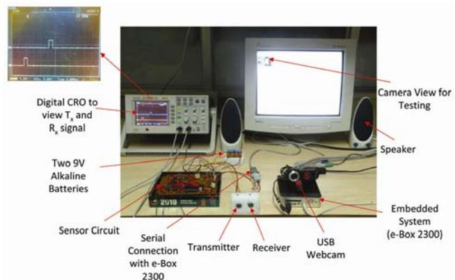
Figure 2. Experimental set-up of the electronic travel aid.
