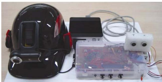
Figure 5. Prototype of the electronic travel aid device.
