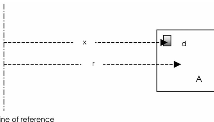
Figure 1. Plane area with reference axis for computation of various moments of area.
